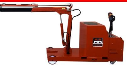
The ATLAS 1TE2 is a full electric powered Pick & Carry crane with a maximum capacity of 1000 Kg and with a double electric boom that reaches a free overhang of 2250mm. One of the key features of this pick and carry crane is that there are no lateral outriggers, therefore this crane grants max mobility with suspended load.
