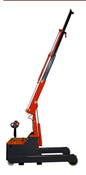
Models OMNIA 2TL and 2TR are a full electric powered Pick & Carry crane with a maximum capacity of 2000 Kg and with a triple electric boom that can reach a free overhang of more than 3 meters.
